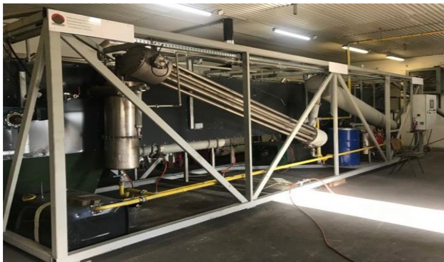
Fig. 1. Installation of waste pyrolytic transformation
